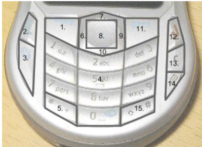
Figure 7: Keycodes and scancodes for phone keys usable from Python applications
