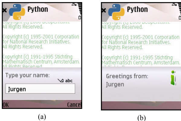
Figure 1. Screenshots of a simple PyS60 application. (a) Text input field; (b) Pop-up note;
